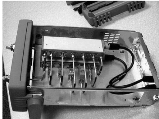
Figure 1-3 The Noise Source Test Set Schematic Component Layout
